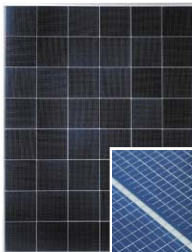
Special: The module is assembled using cells, which have a copper electrode placed perpendicular to the thin silver contact fingers. The bus-bars are next to the cells.
